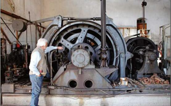
THE ORIGINAL HOIST ENGINE that lifted copper from the depths of the Keweenaw Peninsula ran for years after the Champion Mine was closed in Painesdale in 1967. It was later used to pump water for municipal use by Adams Twp. Newer water pumps eventually replaced it.
